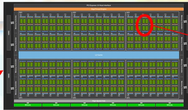
Each GPU has 80+ Streaming Multiprocessors (SMs) and 16 GB of shared memory (HBM2)
