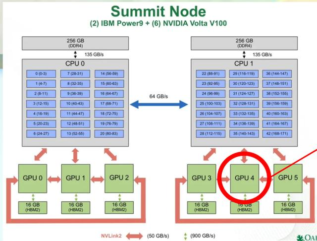
Each Summit node has 6 NVIDIA Volta V100 GPUs. We plan to have 1 ELM MPI task per GPU, so 6 MPI tasks per node
