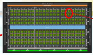
Each GPU has 80+ Streaming Multiprocessors (SMs) and 16 GB of shared memory (HBM2)
