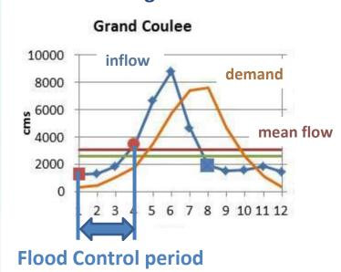
Dam regulation scheme combines flood control and irrigation needs
