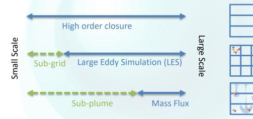
Sub-plume scale effects in ADHOC are included in turbulent flux and mean state equations through generic source/sink term
